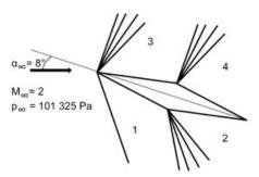
Calculate the lift and drag forces exerted on the airfoil assuming that the chord is equal to 1m (R =287 J/ (kg K),  $\gamma=1.4,~T_{\infty}=188$ K).
